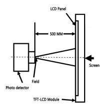
Note 2: Definition of viewing angle range and measurement system. The viewing angle is measured at the center point of the LCD by BM-7A.
