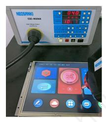
3.1 Electrostatic discharge test
