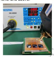
3.1 Electrostatic discharge test
